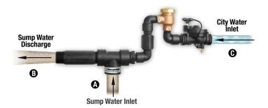
The Basepump with the AVB optional backflow preventer adds an additional level of protection. When a backflow condition occurs, The AVB valve allows air to enter the system, which breaks any siphon effect.
